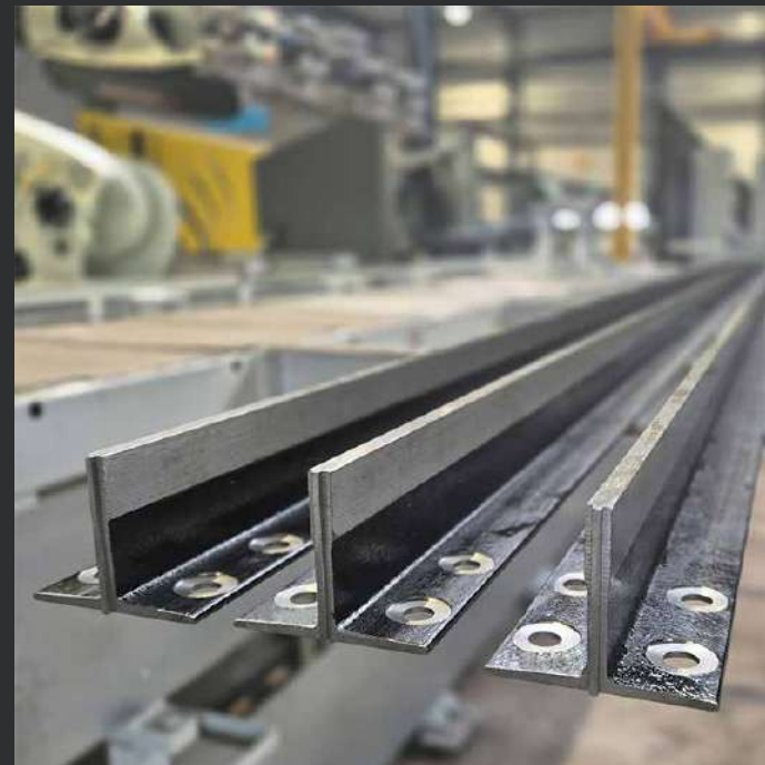
ELEVATOR GUIDE RAILS
